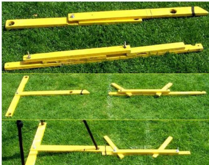
The tactile sighting aid comprises two parts, a stand and the tactile device itself. Stands are typically adapted from photographic tripods, music tripods, or similar. The purpose of the stand is to enable the tactile device to be moved up and down so that adjustments in elevation of the bow can be achieved.
